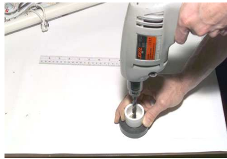
Figures 3.1a and 3.1b. Drill the PVC piping (1/4 in. drill bit) and end cap (3/8 in. bit).
