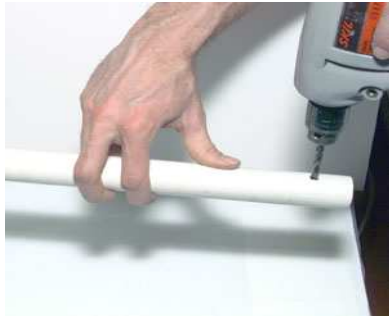
Figures 3.1a and 3.1b. Drill the PVC piping (1/4 in. drill bit) and end cap (3/8 in. bit).
