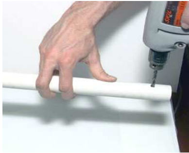
Figures 4.1a and 4.1b. Drill the PVC piping (1/4 in. drill bit) and end cap (3/8 in. bit).
