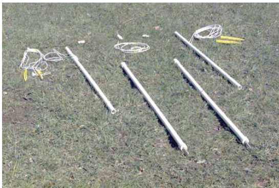
Figure 5.3a and 5.3b. Sample pictures for 10-foot mast setup. Lay out each dipole on the ground and set up one pole at a time.
