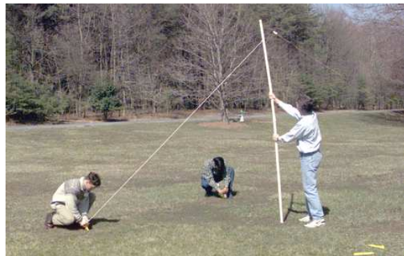
Figure 5.3a and 5.3b. Sample pictures for 10-foot mast setup. Lay out each dipole on the ground and set up one pole at a time.
