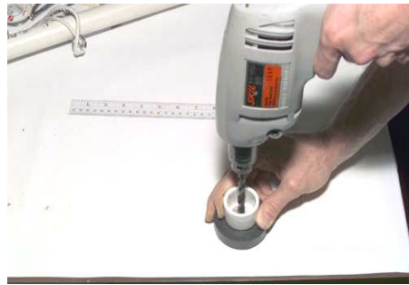
Figures 4.1a and 4.1b. Drill the PVC piping (1/4 in. drill bit) and end cap (3/8 in. bit).
